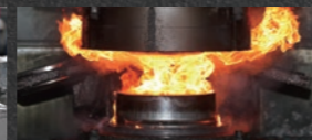
The aluminum alloy is compressed using a high-pressure forging press. During the forging process, the internal grain structure of the metal is finely deformed to produce a material that maintains a high level of strength, even when thinly shaped.
